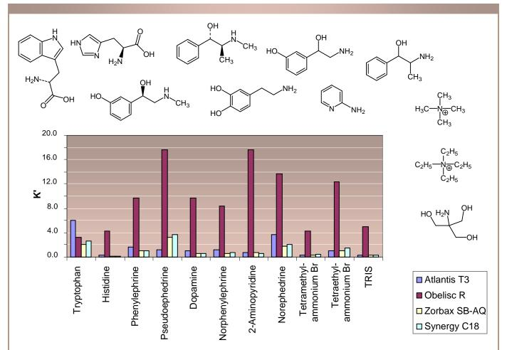
Figure 3. Retention of Polar Analytes on Obelisc R, Atlantis T3, Zorbax SB-AQ and Synergy C18 Columns. Mobile phase: 5% ACN, 20 mmol Ammonium Acetate pH 5
