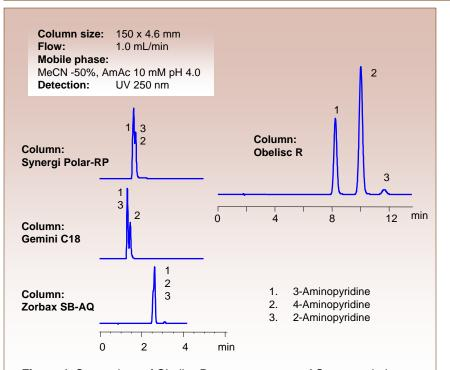
**Figure 4.** Comparison of Obelisc R to some common AQ reversed-phase C18 columns for the separation of aminopyridine isomers.
