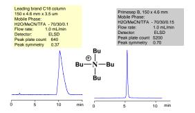
This example shows the effect of a sample diluent on a peak shape of dopamine. When the concentration of the organics reaches 30%, dopamine peak shape and the retention get inconsistent which makes the identification and quantitation impossible.
