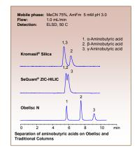
α-, β-, and y-aminobutyric acids are very polar zwitterionic isomers which show little or no retention on reversed-phase C18 columns. These isomers not only retain on Obelisc R and N columns, but they also demonstrate the selectivity available on these columns.
