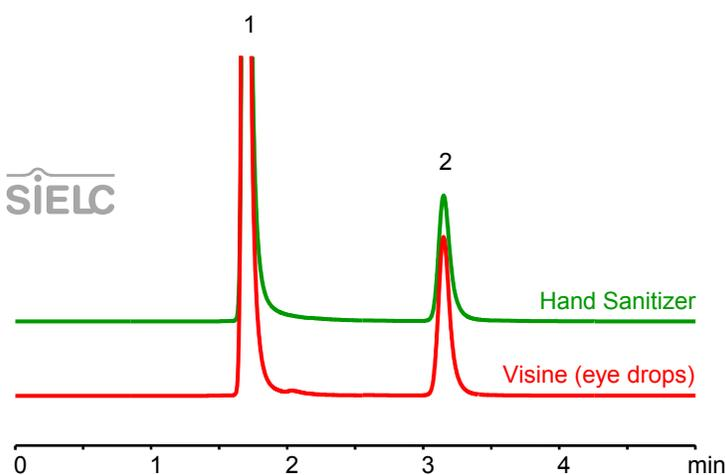
**Fig. 3. Isocratic chromatogram of EDTA complex with Fe(III).** HPLC column: Newcrom BH, 4.6 x 150 mm, 5  $\mu$ m. Flow rate: 1.0 mL/min. Mobile phase: 2% MeCN in water containing 0.1% H<sub>2</sub>SO<sub>4</sub>. Detection: UV 260 nm.
