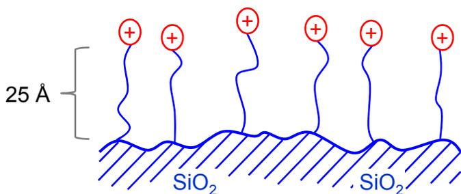
Fig. 6. Schematic structure of Newcrom BH column surface chemistry
