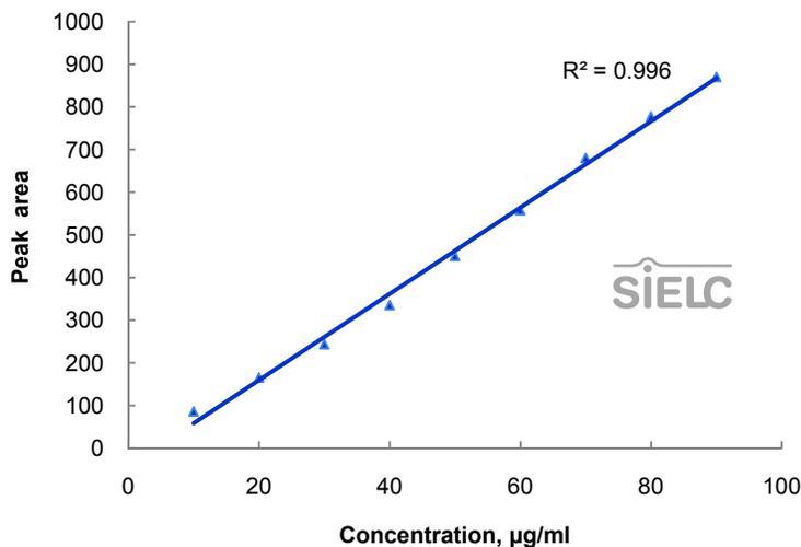
Fig. 5. Linearity study of the EDTA analysis quantitation method. Analytical column: Newcrom BH, 4.6 x 150 mm, 5 µm. Flow rate: 1.0 mL/min. Mobile phase: 2% MeCN in water containing 0.1% H<sub>2</sub>SO<sub>4</sub>. Detection: UV 260 nm. Injection: 5 µL of EDTA standards with FeCl<sub>3</sub> solution.
