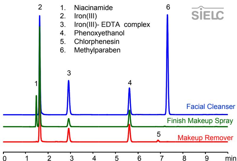
**Fig. 4. Gradient method.** HPLC column: Newcrom BH, 4.6 x 150 mm, 5  $\mu$ m. Flow rate: 1.0 mL/min. Mobile phase: MeCN gradient from 2 to 70% in water in 10 min, mobile phase contains 0.1% H<sub>2</sub>SO<sub>4</sub>. Detection: UV 260 nm. Injection: 5  $\mu$ L of sample.
