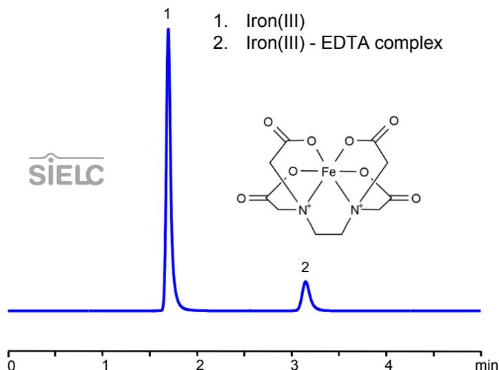
**Fig. 2. Chromatogram of EDTA complex with Fe(III).** HPLC column: Newcrom BH, 4.6 x 150 mm, 5  $\mu$ m. Flow rate: 1.0 mL/min. Mobile phase: 2% MeCN in water containing 0.1% H<sub>2</sub>SO<sub>4</sub>. Detection: UV 260 nm.
