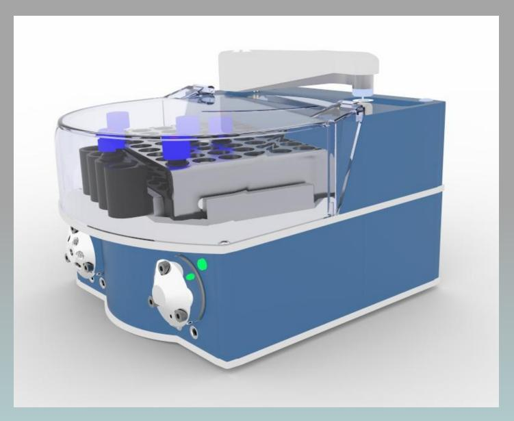
This autosampler application allows to automate sample introduction in a high pressure line for applications such as HPLC (High Performance Liquid Chromatography). Accurate sample volume from 1 to 100  $\mu$ L can be introduced in the high pressure stream without loosing operational pressure. Additional functions includes sample mixing, needle cleaning with up to 4 solutions, sample shaking. Sample storage capacity is 48 vials with 2 mL volume or 96 well plate.
