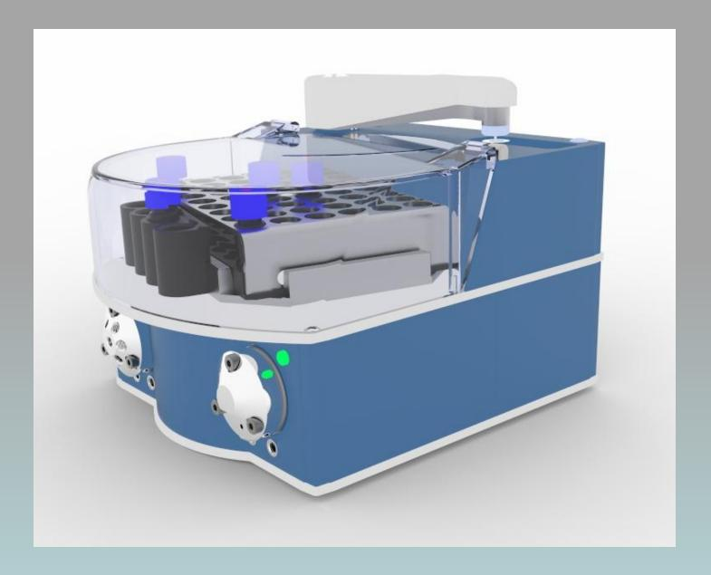
This autosampler application allows to do fraction collection during column chromatography or any other process which produce liquid flow. Fraction can be setup by volume or time. Several tray options are available for different fraction amount. Additional functions includes fraction dilution or mixing with a reagent, needle cleaning, flow diverting.
